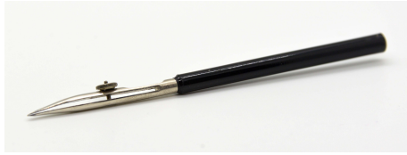
Figure 4.24: A ruling pen, used for technical drawing
